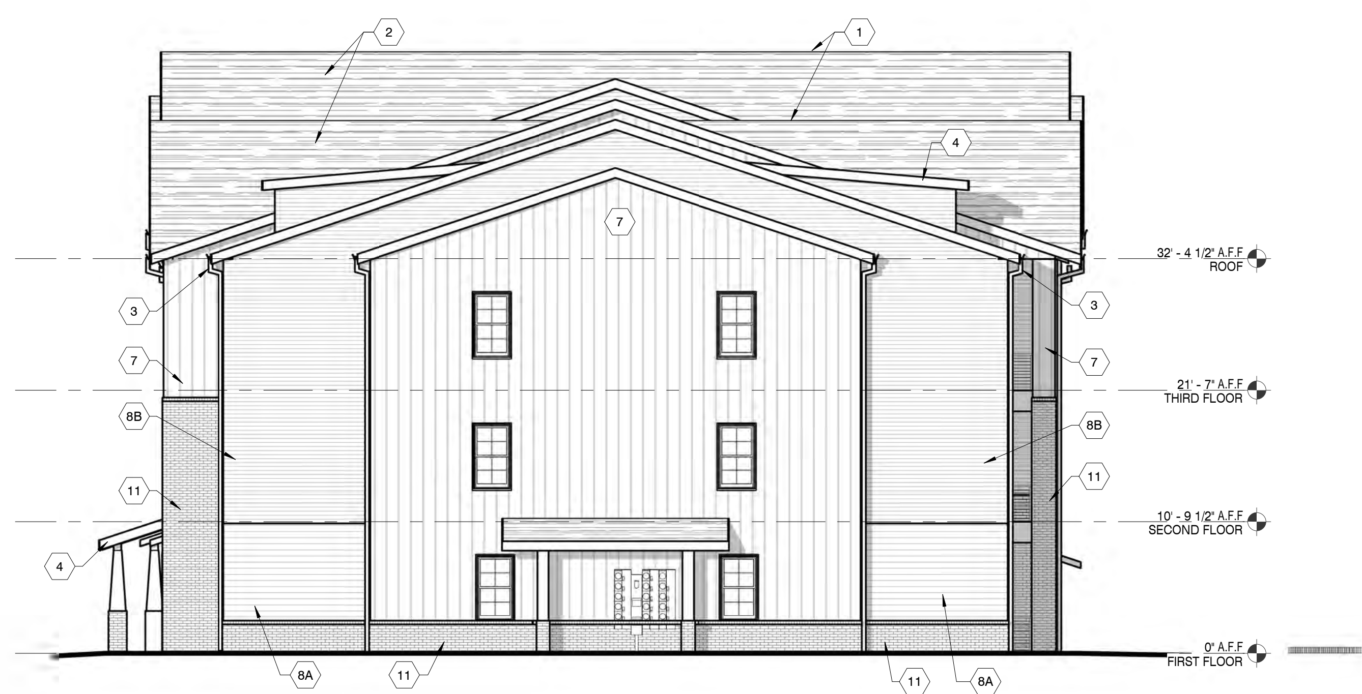
4 BLDG B1 - RIGHT ELEVATION 1/8" = 1'-0"
