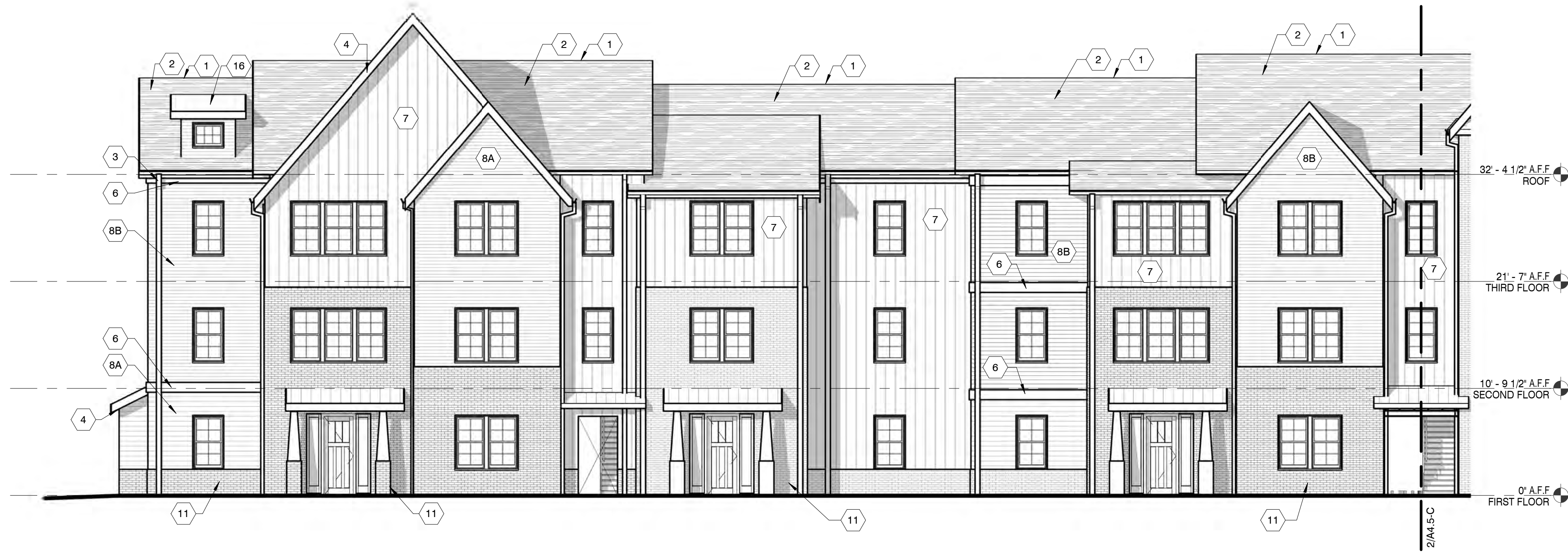
1 BLDG A4 - REAR ELEVATION - PART A 1/8" = 1'-0"
