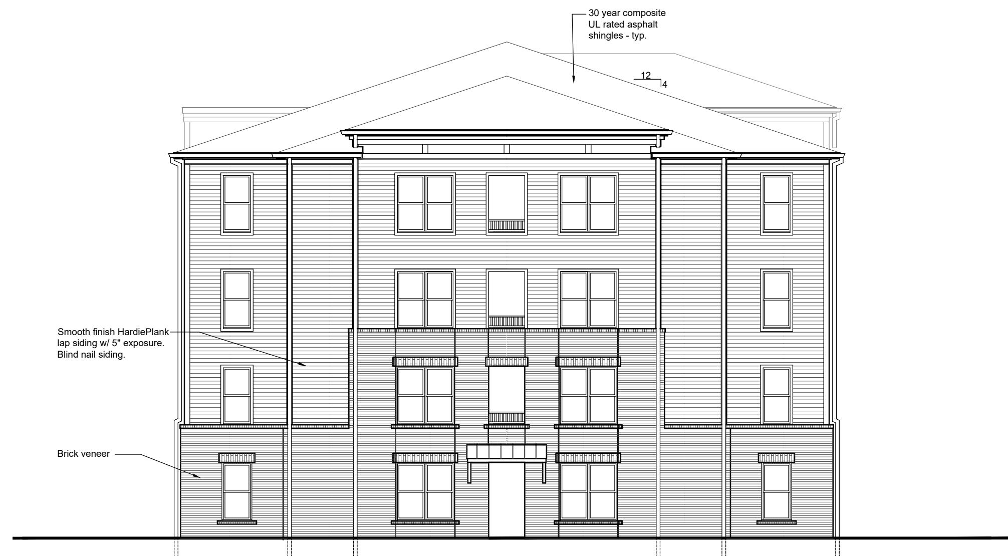
3 Northwest Elevation - (Building 4) Scale: \frac{3}{32} " = 1'-0"
