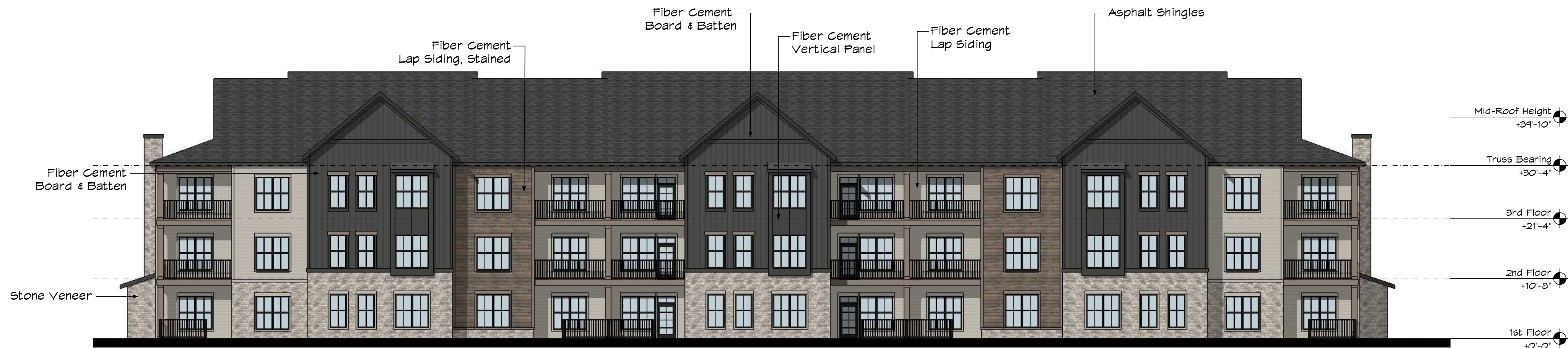
BACK ELEVATION - BUILDING TYPE B Scale: 3/32" = 1'-0"
