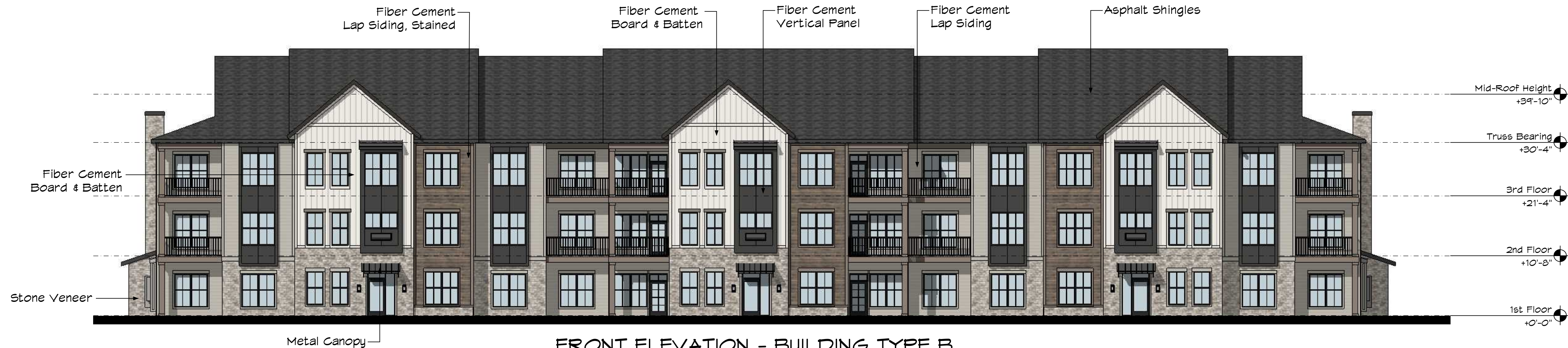
FRONT ELEVATION - BUILDING TYPE B Scale: 3/32" = 1'-0"
