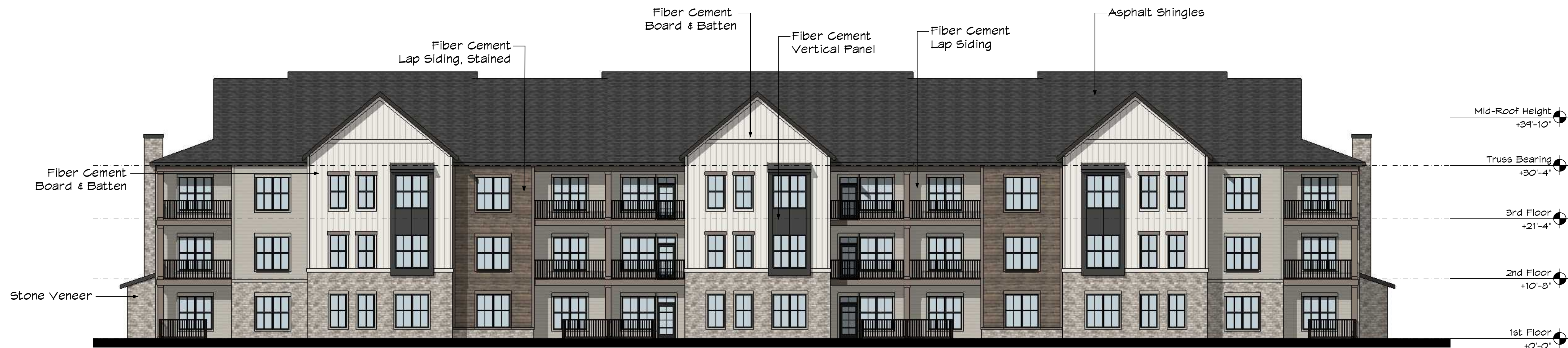
BACK ELEVATION - BUILDING TYPE B Scale: 3/32" = 1'-0"
