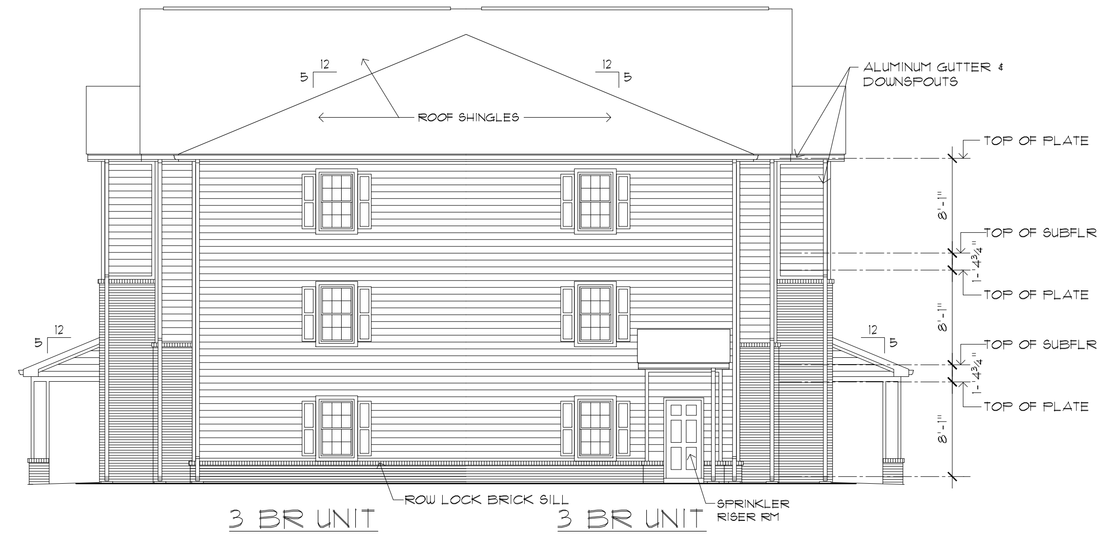
BUILDING A & B - LEFT ELEVATION
