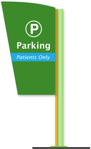
LOCATION J DOUBLE SIDED, NON-ILLUMINATED POST & PANEL SIGN 36" x 22 1/2" PANEL
