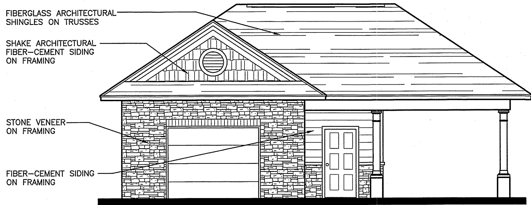
2 MAINTENANCE/CAR WASH FRONT ELEVATION 3/16"=1'-0"
