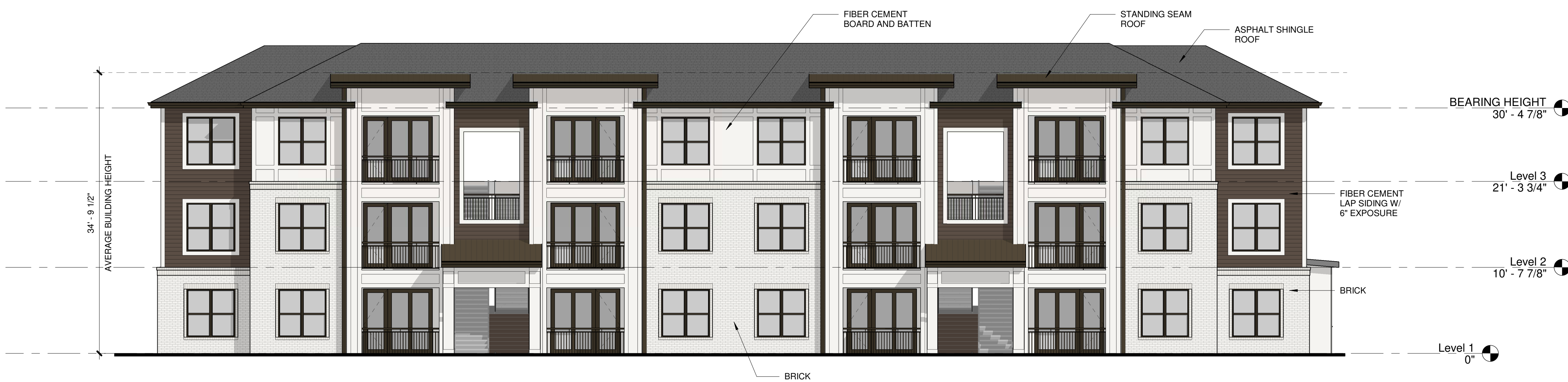
③ BLDG. A SOUTH ELEVATION 1/8" = 1'-0"
